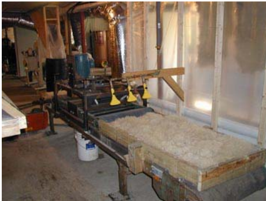
Figure 12. Clean wool about to run under the water jets and into the felting machines, where it is vibrated and rubbed together, causing the separate fibers to cling together in a felted mat.
