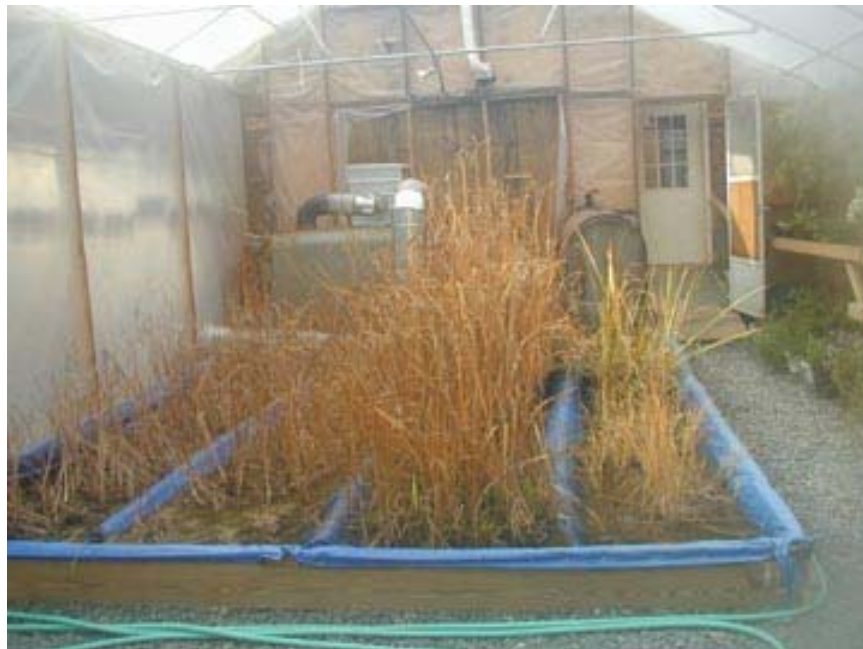
Figure 10. The greenhouse adjacent to the barn, where plants are grown with water from the scouring process. The nursery plants benefits from the “organic waste” eliminated from wool. The center area grows wetland plants (mostly cattails) whose roots are used to “polish” water to its original level of cleanliness, at which point it is recycled to the pond for use in additional scouring.
