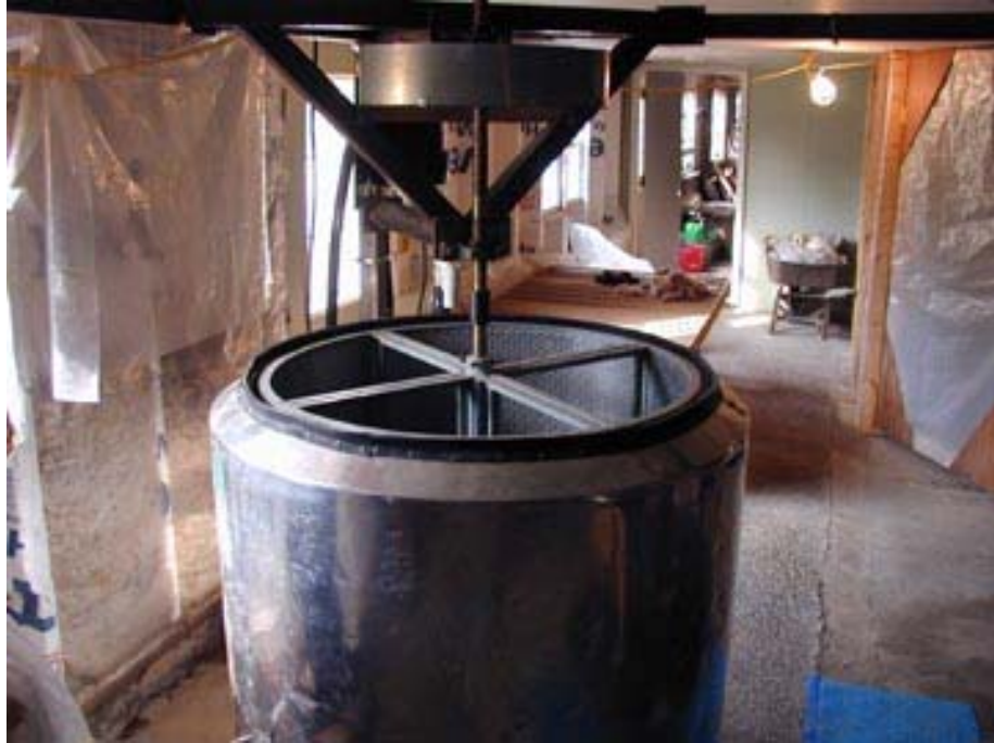
Figure 5. Customized scouring vessel made from an old pasteurizer. Separate sections can segregate wool of different growers, and still allow a single washing to conserve energy and water.
