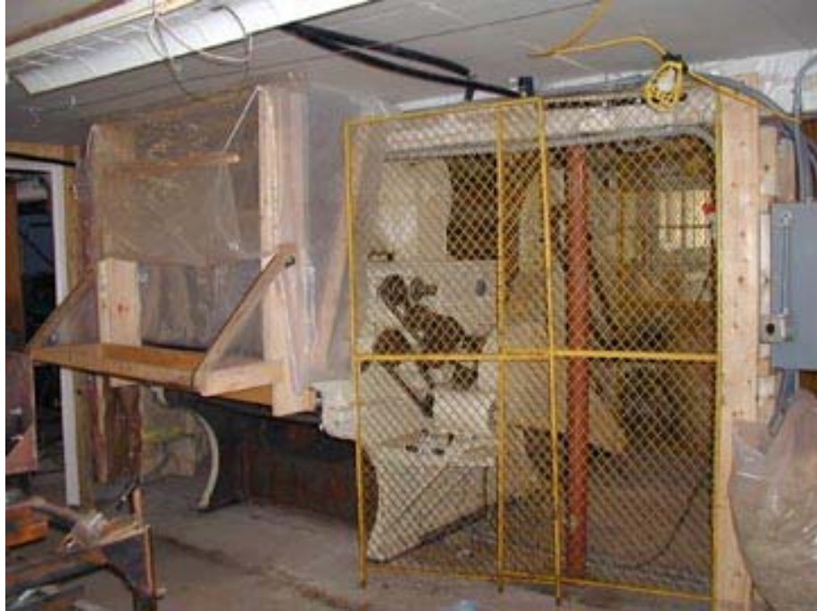
Figure 3. Side view of picker exit, where wool is collected after it has been “picked” clean of any vegetable matter that remained after washing.
