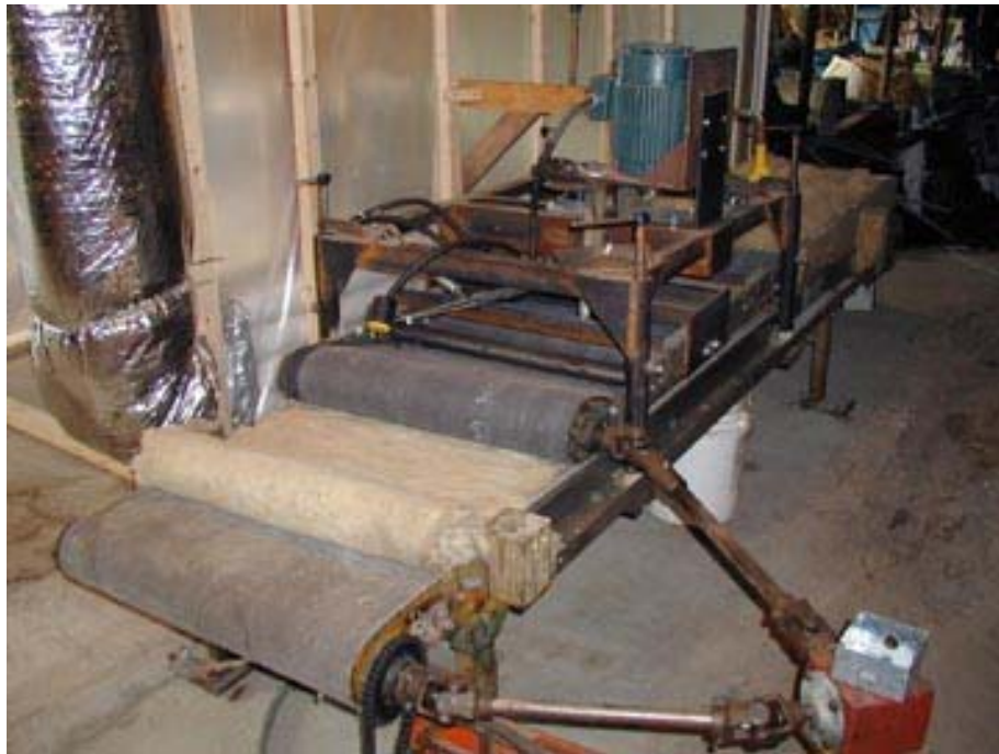
Figure 4. Side view of felting machine with a 2-foot width of felted wool weed barrier on equipment.
