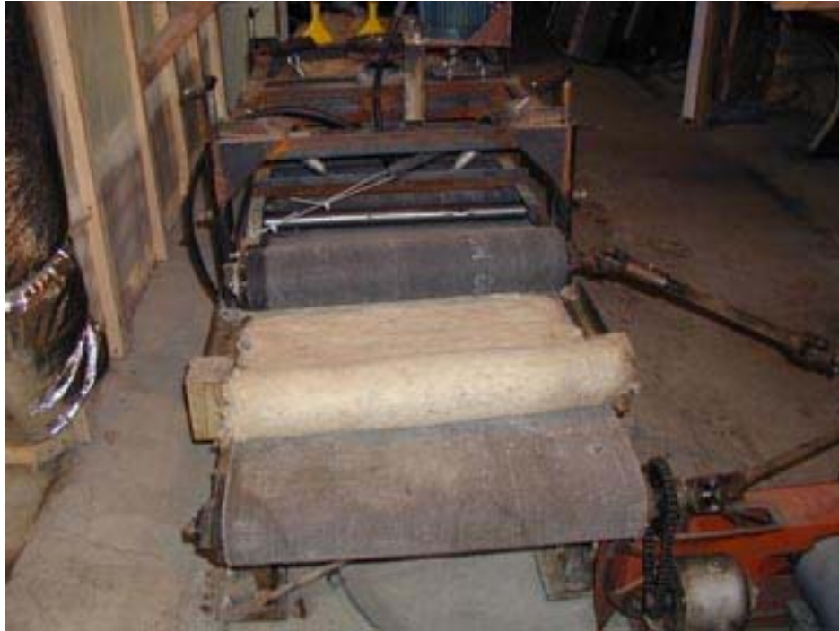
Figure 13. A roll of felted weed barrier at the finished end of the felting machine.
