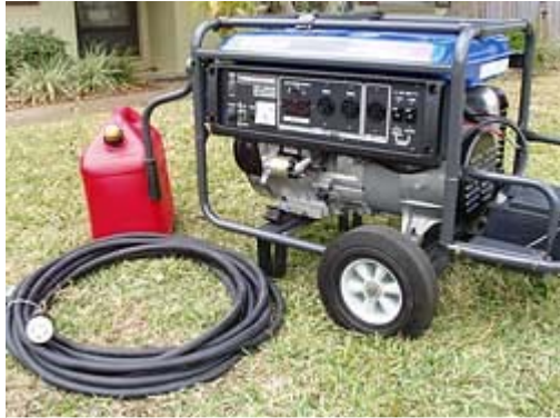
Due to the limited fuel tank size on many small generators and their rate of fuel consumption, users are often required to refuel generators several times a day.
